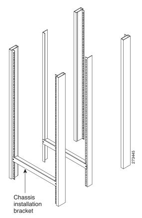
**Step 4** With two people, lift the chassis (partially unloaded) into position between the rack posts and rest it on the chassis installation bracket.
